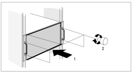
Figure 8: Mounting the basic unit
